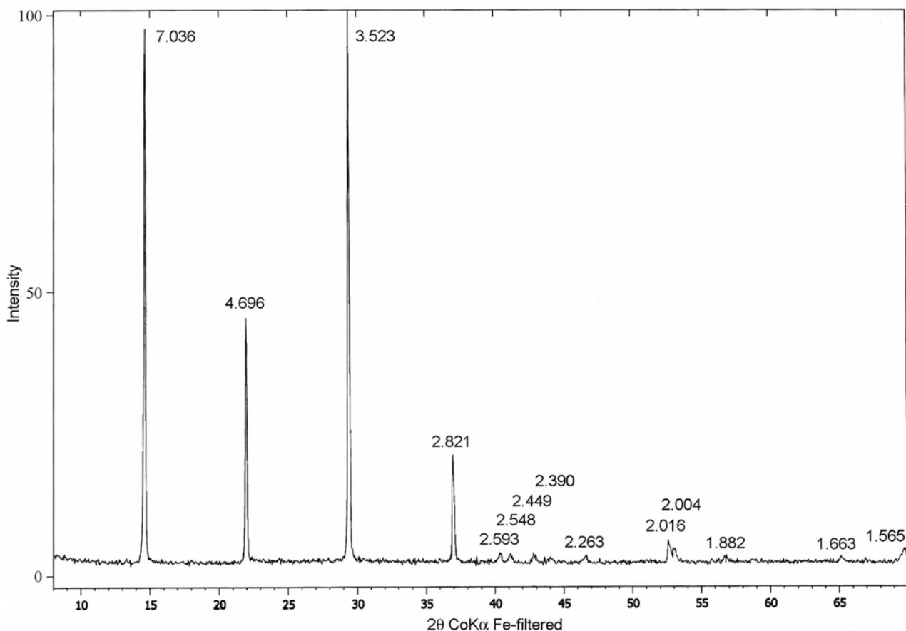
Fig. 2. X-ray diffraction pattern of powder sample from the studied stone tobacco pipe
