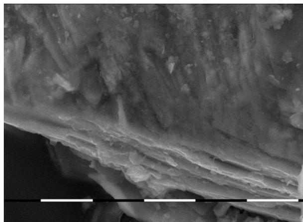
Fig. 5. Perfect cleavage along the basal pinacoid of the studied chlorite; scale bar 10 µm
