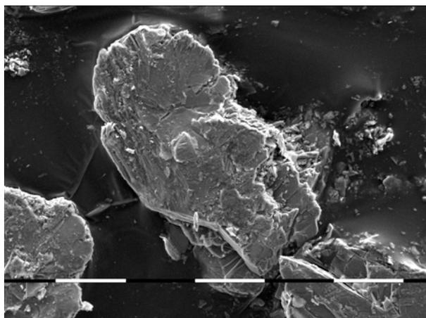
Fig. 4. Chlorite aggregate from the studied stone tobacco pipe with entrance and inner angles characterizing a pseudo-hexagonal habitus of the chlorite flakes; scale bar 10 µm
