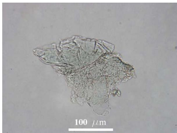
Fig. 3. Flaky habitus of chlorite aggregate from the studied stone tobacco pipe in optical microscope, //N
